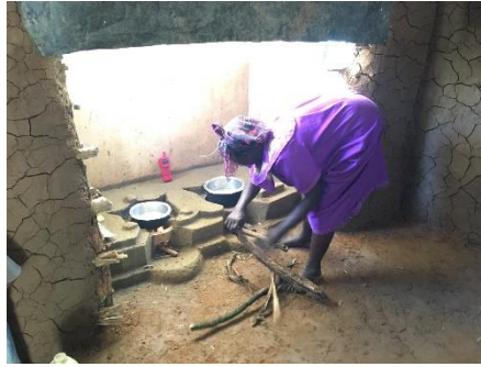
Fig. 7. Interior view of prototype kitchen showing easy access to the stoves from the inside of the kitchen.
